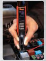
THE TOP OF THE TOOL SHOWS INACTIVE, ACTIVE, OR OPEN FOR QUICK FUSE DIAGNOSIS.
